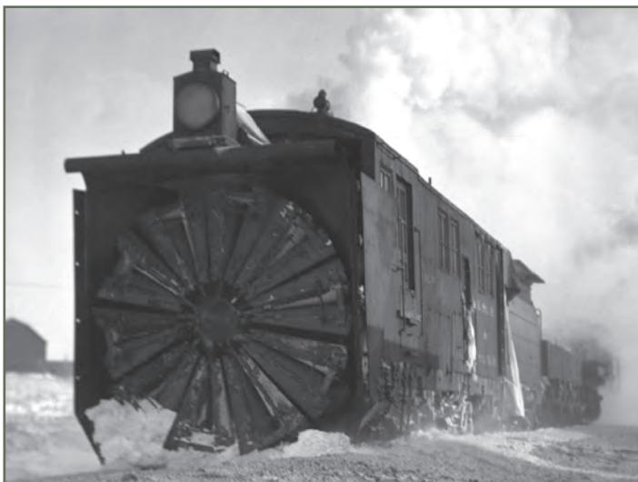
Close up of a rotary snowplow on a train near Kenmare, ND, in 1916. SHSND SA 2012-P-064-001276
